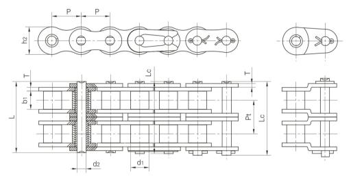
双排滚子链/套筒链 Duplex roller chains & bushing chains
